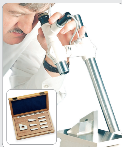
Figure 8: Autocollimator being used to compare manufactured prism against a master angle gauge
