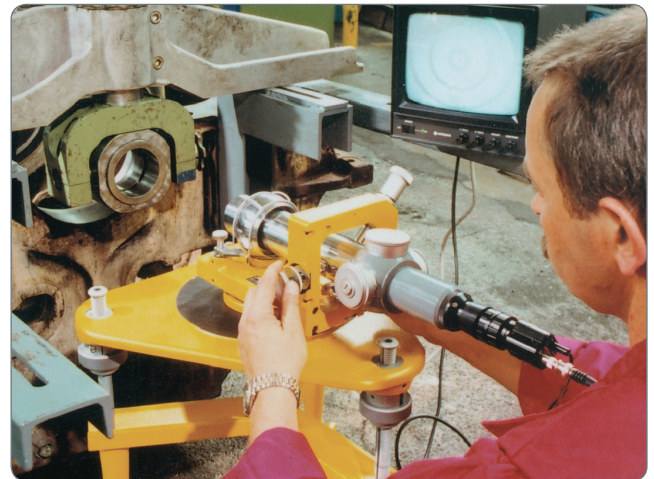
Alignment of bearings in a large diesel engine prior to machining of bore
