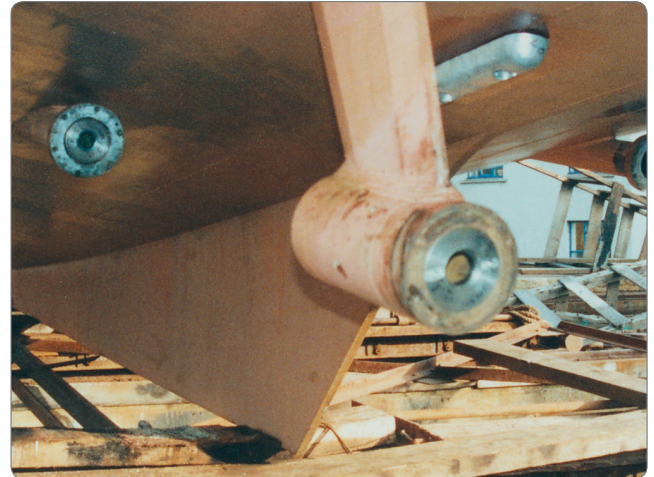
Checking the alignment of the engine/gearbox, propellor shaft bearings and 'P' bracket bearings
