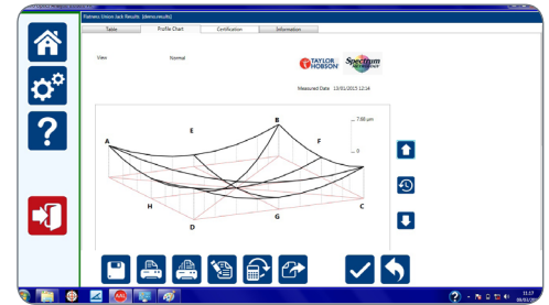
Figure 2: Surface plate generators (picture from software measurement screen for Union Jack)
