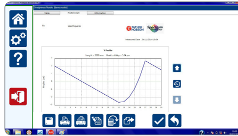
Figure 5 – Graph from computerised straightness check
