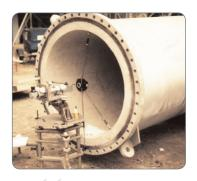
Taylor Hobson's Micro Alignment Telescope is ideal for checking perpendicularity and parallelism of pipe and tube end faces in industry.
