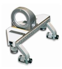
Among the large number of applications possible with the Taylor Hobson Autocollimator, the most common is the simultaneous two axis straightness measurement of machine tool slideways.
