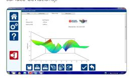
The results are displayed in tabulated form. Deviations from straightness in both axes are given as maximum peak and minimum valley values, and the appropriate step number indicated. The out of straightness is the maximum peak to valley and can be calculated using either the ends zero or least squares method.
