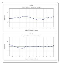
A Talyvel electronic level is used in conjunction with the autocollimator to measure the twist or roll of the slideway.
