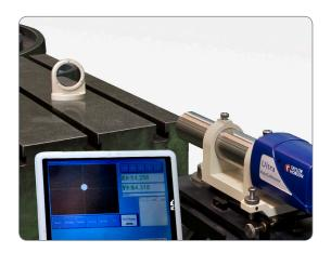
Ten-metre slides can be checked in a few minutes, with automatic measurements taken at X and Y directions along the slideway.
