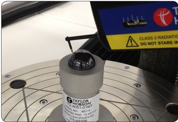
Fig. 3: PGI Dimension measurement of R12.5 mm calibration standard – traverse unit tilted at 30 degrees.
