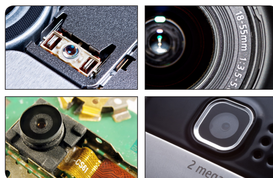
Figure 2: Common applications of steep-sided miniature aspheres
